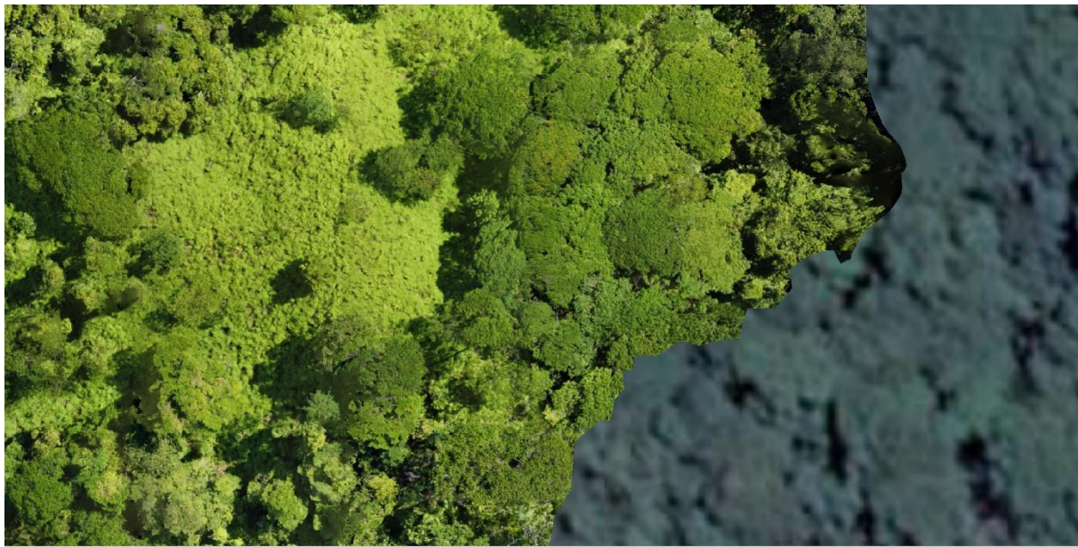
Figure 5: Part of a processed image embedded in QGIS. The left side of the image shows the drone imagery while the right side shows the underlying satellite image. The fern dominated area is reflected in a light green from the left side to the centre. Source of Satellite image: Google Earth. (05.03.2015). La Gamba, Costa Rica. © 2022 CNES / Airbus.
